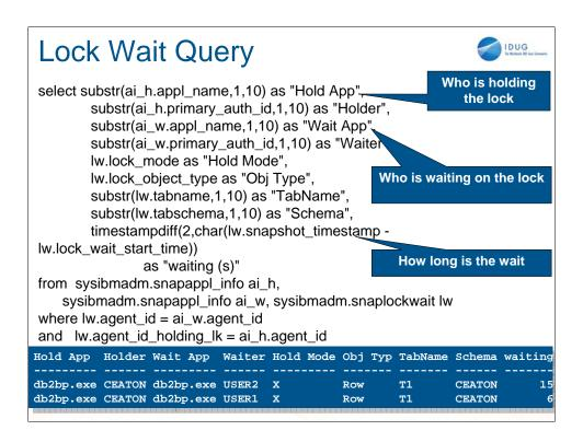
This query shows you any lock chains that currently exist. It shows the lock holder, the application/user waiting on the lock as well as the object locked and the length of time the waiter has been waiting. It is not abnormal to see lock wait chains. What is abnormal is to see lengthy waiting times. If you see long waits, you should look at what the holding application is doing (what SQL statement and what the application status is) to determine if the application is well tuned.
